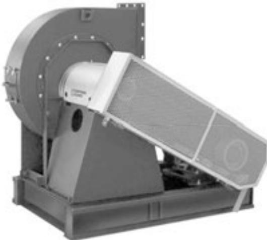
Rotatable housing can be field rotated to the standard discharge positions shown in the Series 6600 Drawing Supplement (Bulletin 6600-1). The field reversible feature allows for the wheel and housing to be removed in the field and reversed, along with a change in discharge. This feature is only available on Design 6610 since the impeller can be run in either clockwise or counter-clockwise rotation.
