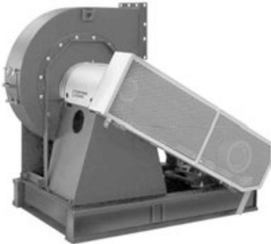
Rotatable housing can be field rotated to the standard discharge positions shown in the Series 6600 Drawing Supplement (Bulletin 6600-1). The field reversible feature allows for the wheel and housing to be removed in the field and reversed, along with a change in discharge. This feature is only available on Designs 6610 and 6620 since the impellers can be run in either clockwise or counter-clockwise rotation.
